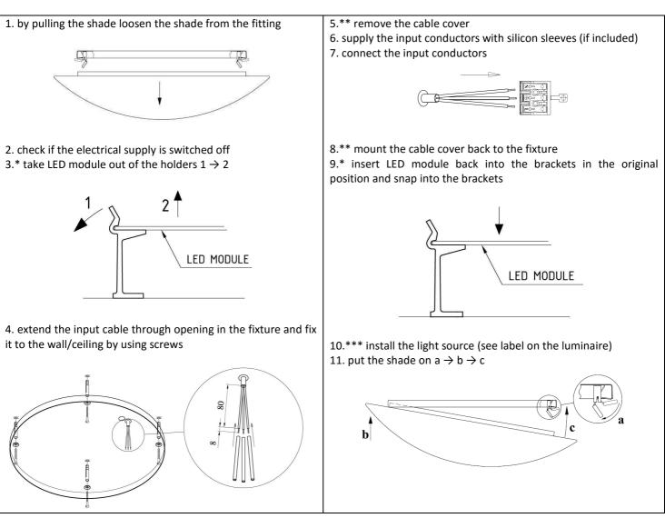
\* Apply when install lights with LED module Osmont (for example L12, L13, L32, L43 ...). CAUTION when handling the LED module and feeder cables to the LED module! Do not touch the LEDs!
